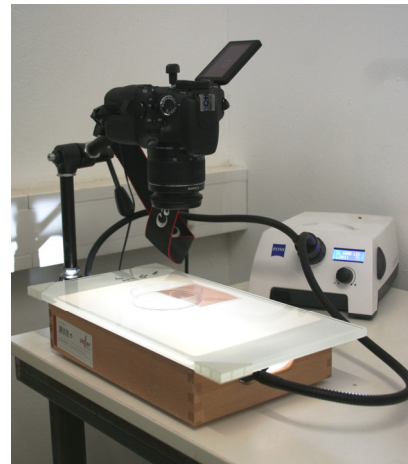
Figure 1. Experimental setup including light table, camera and light device.
